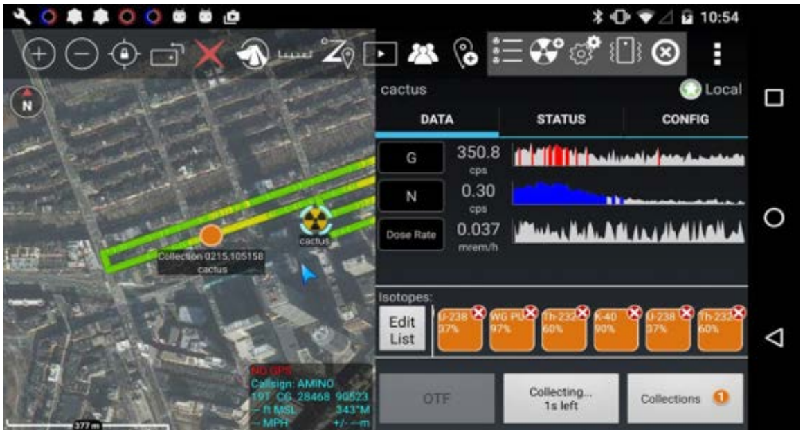
Figure 2. Example of the RN plugin for ATAK, showing connection to a radiation sensor with gamma and neutron detection capability, count rates for each radiation type plus dose rate, and a map with heat indicators proportional to dose rate.
